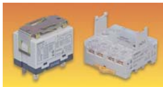
Relay with mounting bracket fitted L=52.5, W=33.5, H=47 (53 with 472-530 fitted) Terminals: 6.35 x 0.8 x 11
